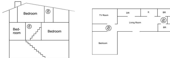
In homes with more than one sleeping area, a smoke detector (indicated by an inverted "s" in a circle) should be provided to protect each area.
