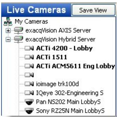
Drag and drop the desired cameras from the camera tree on the left side of the screen to the Video Panel. You can replace the video in a panel by dragging a new camera in from the camera tree or from another panel. Note that you can drag and drop cameras from any networked exacqVision server that you can connect to, regardless of where it is located.
